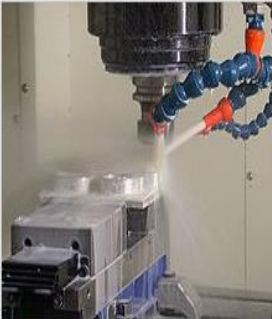
Thin wall milling of aluminum using a water based cutting fluid on the milling cutter
