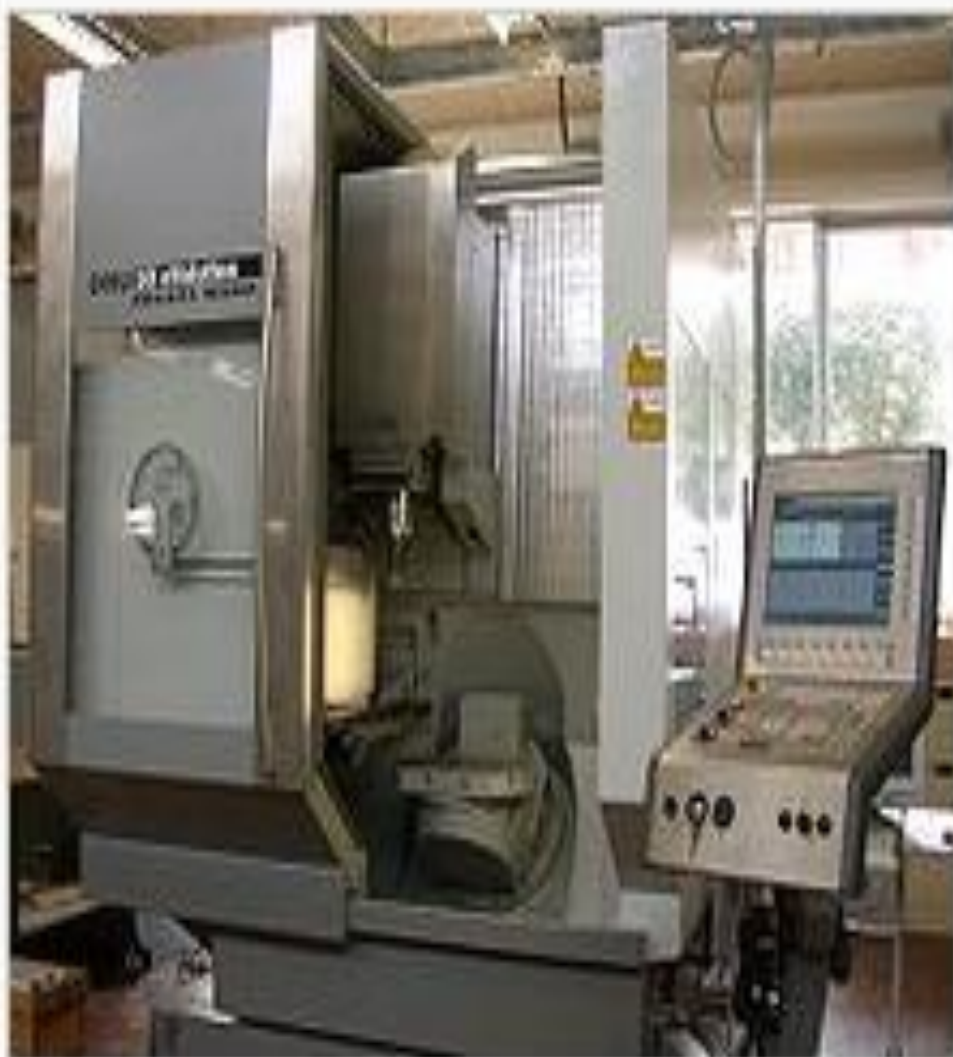
Five-axis machining center with rotating table and computer interface
